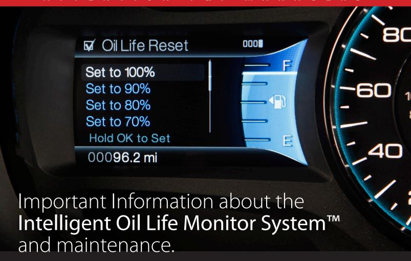
Beginning with the 2011 model year, most Ford and Lincoln vehicles are equipped with an Intelligent Oil Life Monitor™ (IOLM) that determines when the engine oil should be changed based on vehicle operation.
